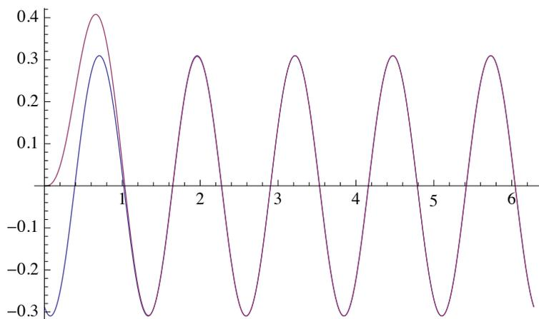
3.6.18. Consider the mass-spring-dashpot system  $mx'' + cx' + kx = F_0 \cos \omega t$  with  $m = 1$ ,  $c = 10$ ,  $k = 650$ , and  $F_0 = 100$  (in mks units). Find and sketch the amplitude  $C(\omega)$  of steady periodic oscillations with frequency  $\omega$ , and find the practical resonance frequency  $\omega$ , if it exists.
