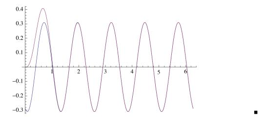
3.6.18. Consider the mass-spring-dashpot system  $mx'' + cx' + kx = F_0 \cos \omega t$  with m = 1, c = 10, k = 650, and  $F_0 = 100$  (in mks units). Find and sketch the amplitude  $C(\omega)$  of steady periodic oscillations with frequency  $\omega$ , and find the practical resonance frequency  $\omega$ , if it exists.
