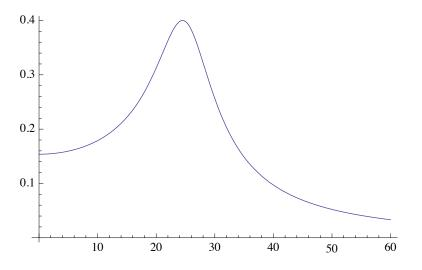
3.6.28. As indicated by the cart-with-flywheel example discussed in this section, an unbalanced rotating machine part typically results in a force having amplitude proportional to the square of the frequency  $\omega$ .
